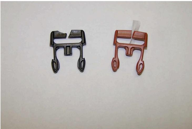
Above are two clips that are modified. The left one has had a section removed from the cross bar. The right has a cut through the cross bar. The modification in both cases was done with shears.
