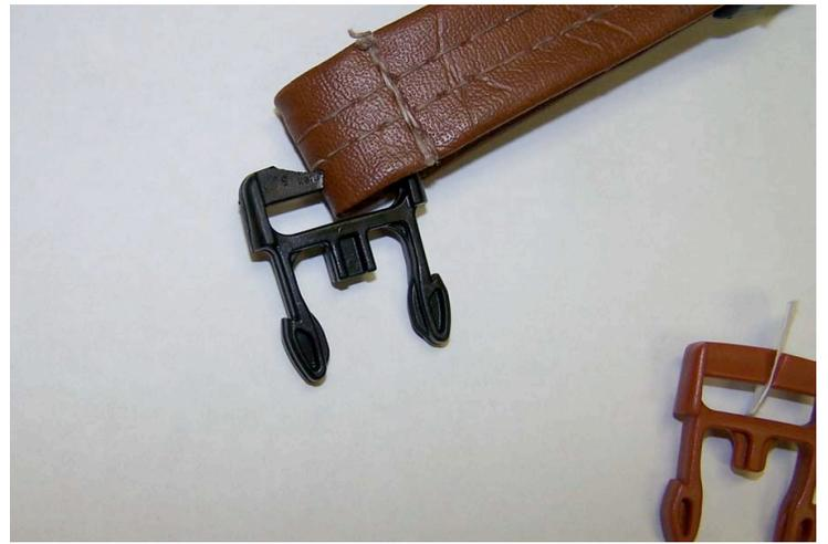
The above picture shows the vinyl strap being inserted through the cut in the plastic of the clip. Further efforts are needed to position the clip on the handle. With a little patience and effort it can be done. It is more difficult to do this on the clip with a simple cut through the crossbar, but that too can be done.
