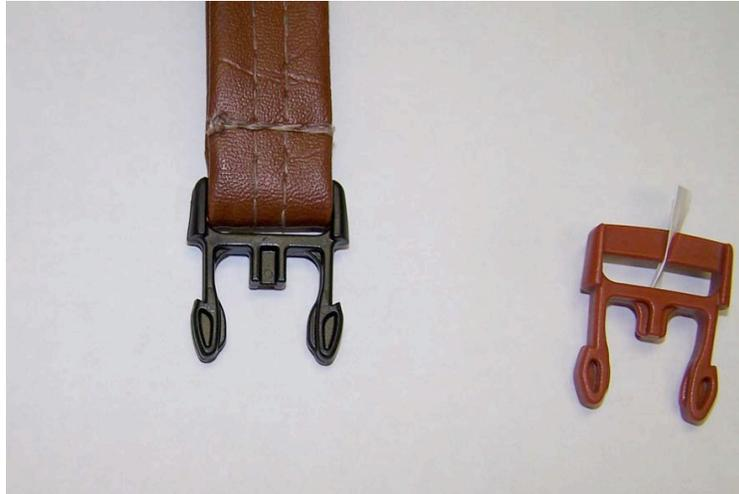
On the left hand side of this picture above is how the clip looks attached to the vinyl spa cover strap. On the right hand side of this picture above is a clip that has been modified to use to repair a broken clip. The top crossbar has been cut.
